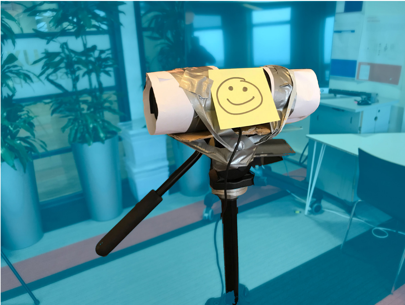
Fig.2 Crude prototype of the conversational lamp-post - loudspeaker on a tripod
